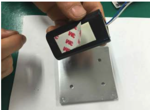
Remove peels of the tape from the new battery pack. And center it carefully on the two holes and make little space between two batteries.
